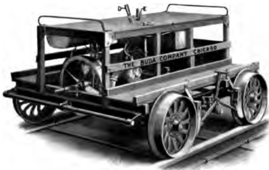
Buda No. 19. Section Motor Car
